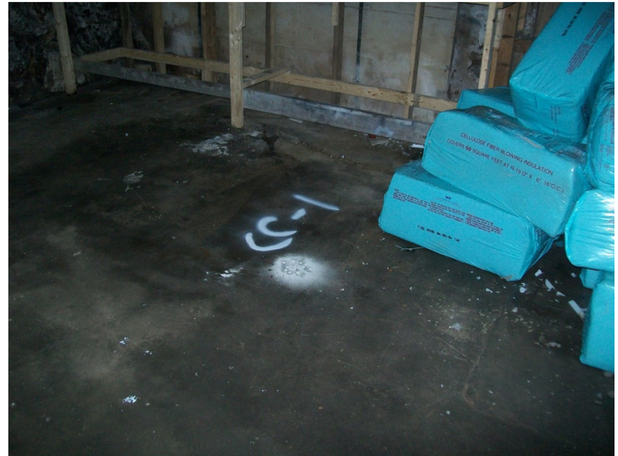
Picture 2 – location of concrete sample CC-1 in garage, where PCBs were identified in concrete
