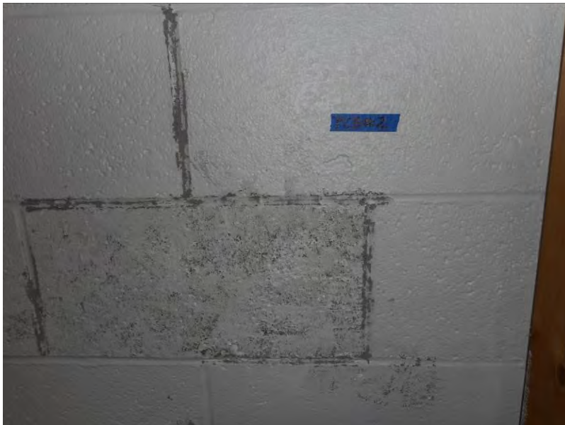
15. Location of CA-PCB-2 collected from white interior paint in the retail store.
