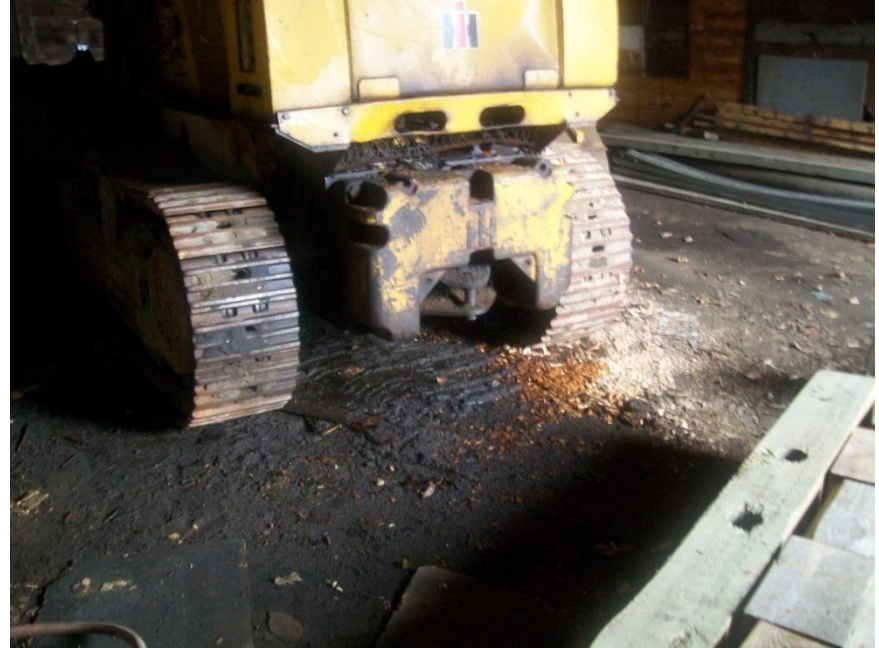
Picture 6 - View of the oil stained soil within the Blacksmith Shop, specifically, oil staining emanating from beneath a bulldozer
