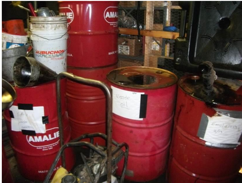
9. Pooled oil on top of drums in the drum storage area.
