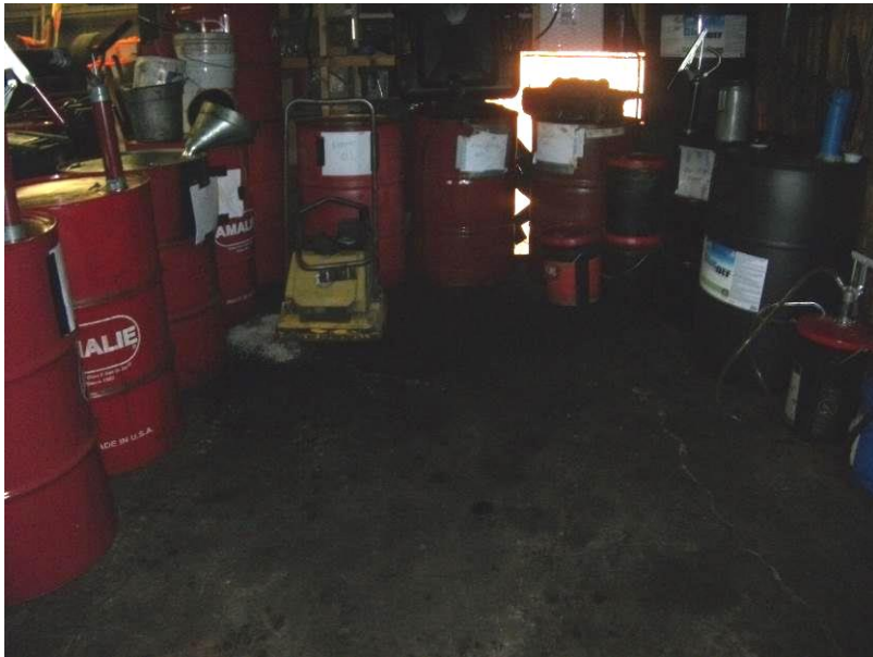
7. Drum storage area within Site building. Note the floor staining.
