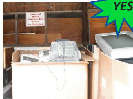
This CRT storage area is protected from weather and properly signed. CRT units are properly contained, ready for transport.
