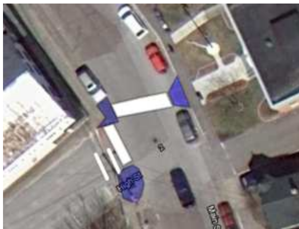
Fig. 24 – Intersection in Meredith where corner bulb-outs could improve pedestrian and driver visibility.
