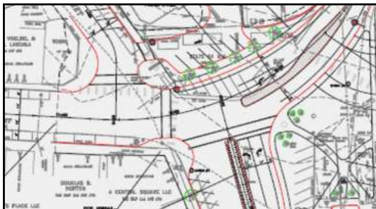
Fig. 16 - Bristol Village enhancement plan showing bulb-outs that shorten crossings, tighten turning radii, and calm traffic.
