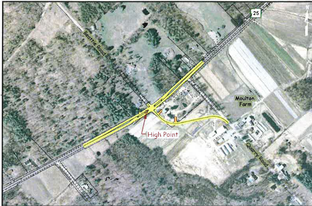
Figure 3.51 – Quarry Road Re-alignment
