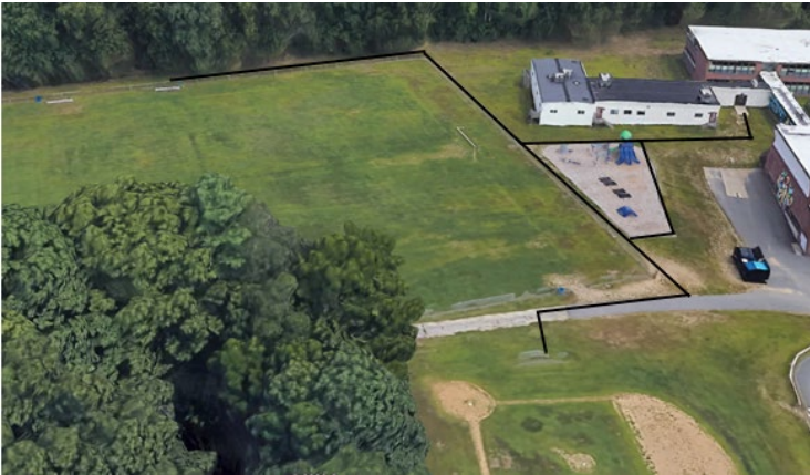
Figure 1: Possible accessible asphalt route from door 9 to and around the playground, and to the team seating and the edge of sport activity at the baseball and soccer fields. (Based on 4’ wide min. x 825’ long asphalt route with a max. running slope of 1:20 (5.00%) and a max. cross slope of 1:50 (2.00%)).
