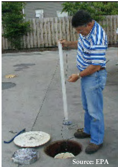
Ground water monitoring of UST secondary containment
