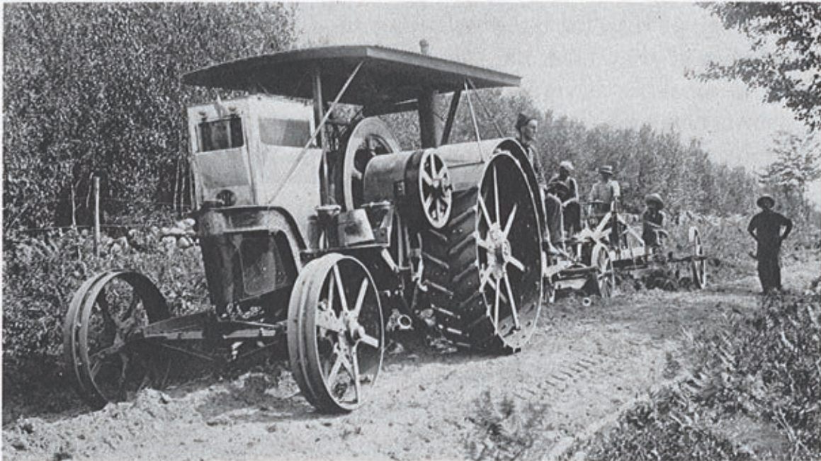
The old steam powered road machine used many years ago to maintain the town's many miles of roadways.
