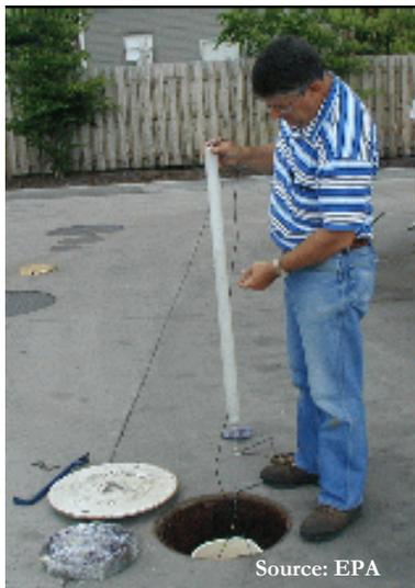
Ground water monitoring of UST secondary containment
