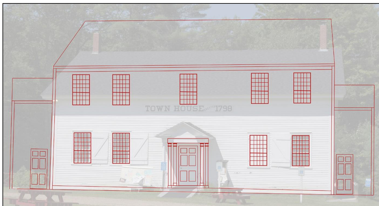
Figure 26: Conjectural drawing of south elevation of New Hampton Meetinghouse in 1798 superimposed on 2022 photograph of New Hampton Town House
